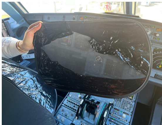
(fig.1) Damage observed on the RH sliding window and on the sunshade (pictures from the Operator)
