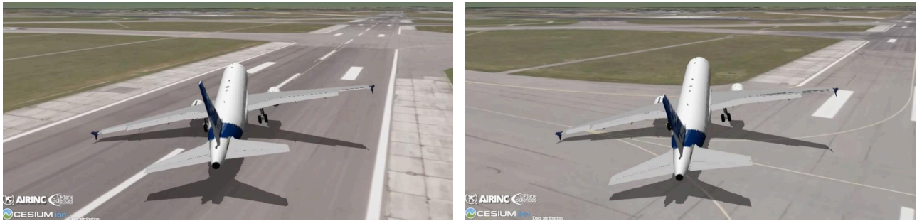
(fig.5) Screen captures from the video reconstruction of the event showing the aircraft attitude in the early stage of the go-around phase (Flight Animation System from APS Aerospace)
