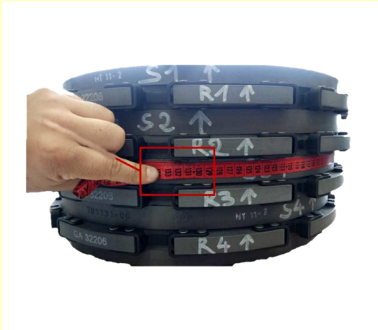
(fig.7) Optional inspection to measure the perimeter of the central stator on Safran Landing Systems and Messier-Goodrich brakes
