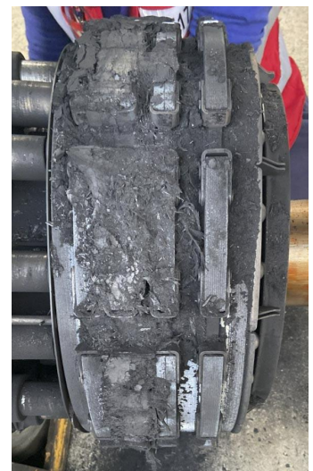
(fig.4) Heavily oxidized brake disks
