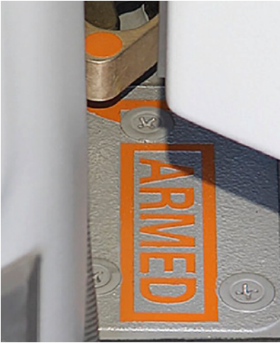
(fig.3) Girt Bar Floor Indicator on A320 Family aircraft
