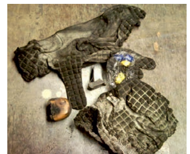
Figure 2 Foreign objects found in an APU compartment
