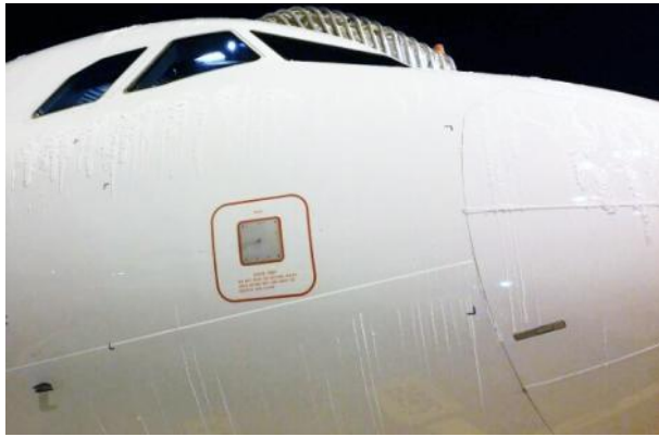
(fig.3) Example of thin ice ridges forward of the Pitot probes of an A320 family aircraft
