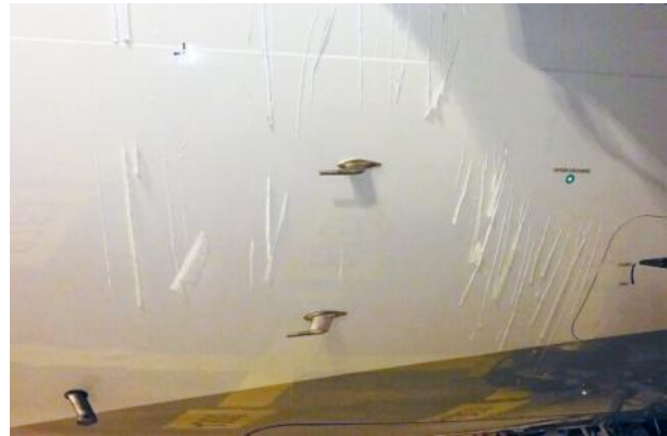
(fig.4) Example of ice ridges that remain on the lower fuselage even after completing a flight
