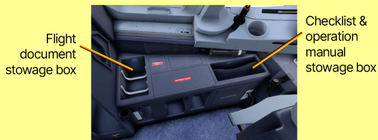
(fig.10) Stowage available in the left hand lateral console of an A320 family aircraft
