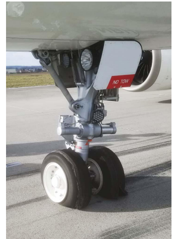
(fig.3) View of the NLG after landing
