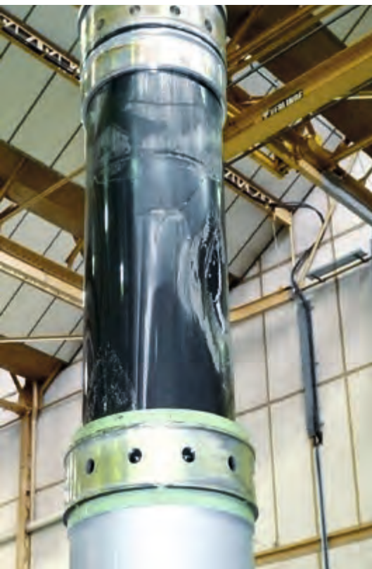
Figure 3 Damage on the aircraft following the hard landing: aircraft's Landing Gear
