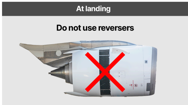
(fig.12) Thrust reversers must not be used at landing
