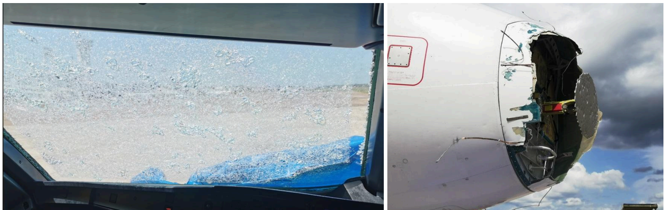
(fig.2) View of the damaged windshield and radome after the event (photos: Investigation Board)
