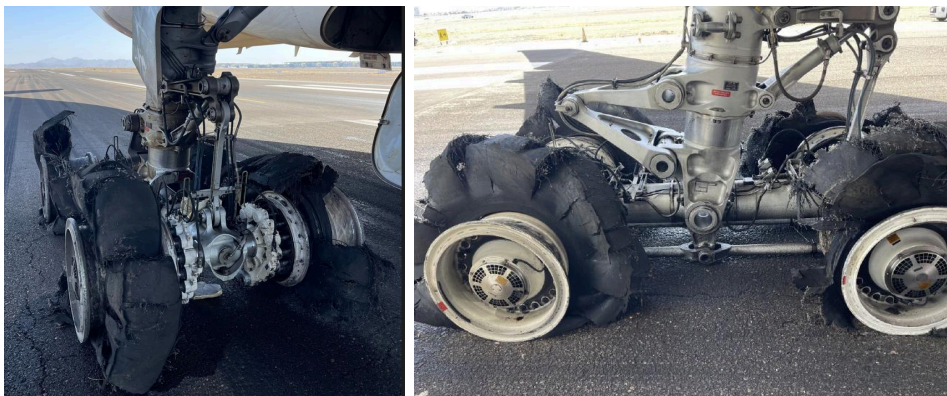
(fig.1) All wheels of the main landing gear burst during the event (images from the investigation board)
