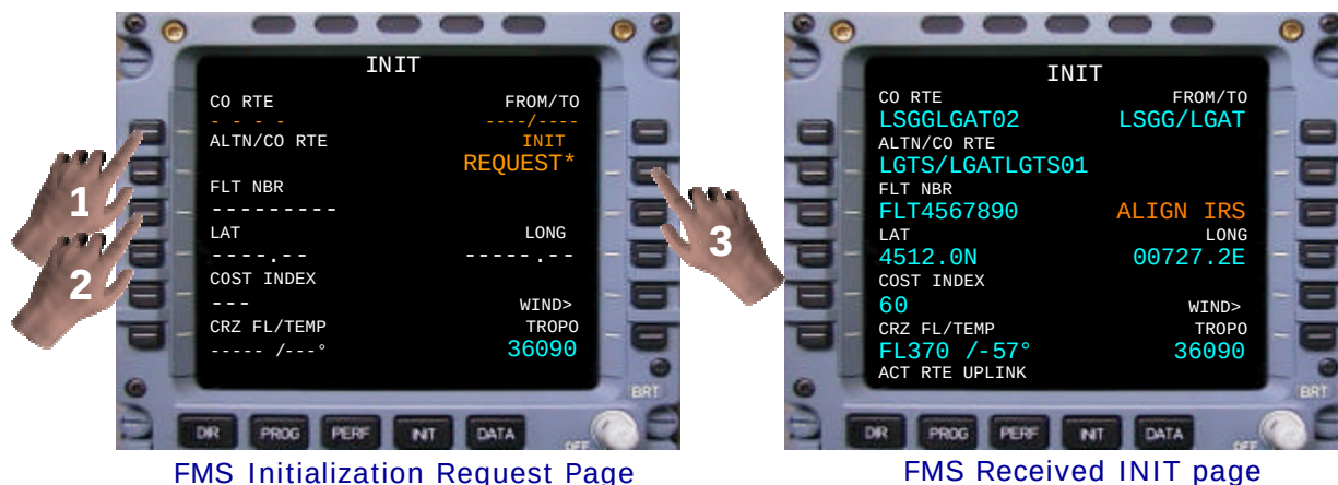
Figure 4.4: Example of FMS initialization MCDU pages
