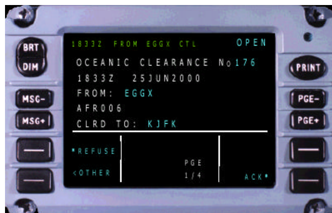
Figure 4.34: Example of Oceanic Clearance with FANS A+ package
