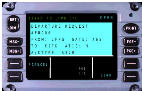
Figure 4.32: Example of DCL request on DCDU (FANS A+ option)
