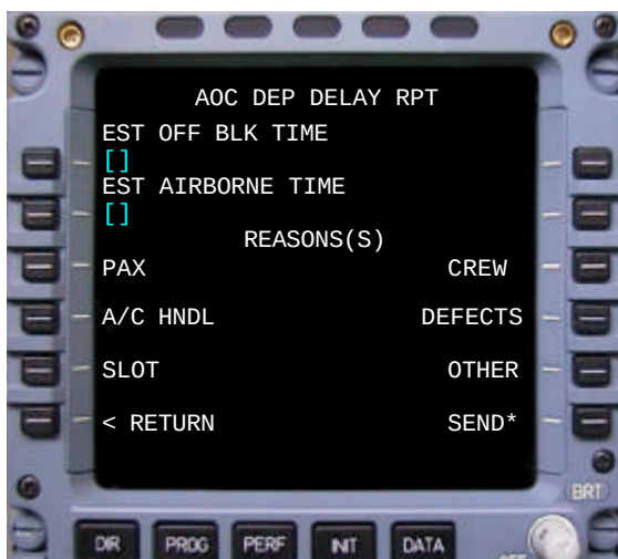
Figure 4.7 Example of departure delay report MCDU screen
