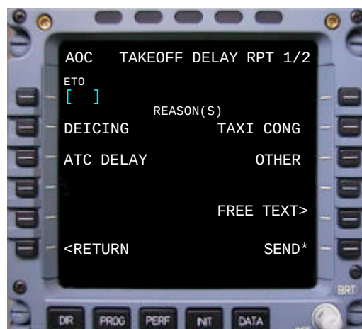
Figure 4.9: MCDU Takeoff delay page
