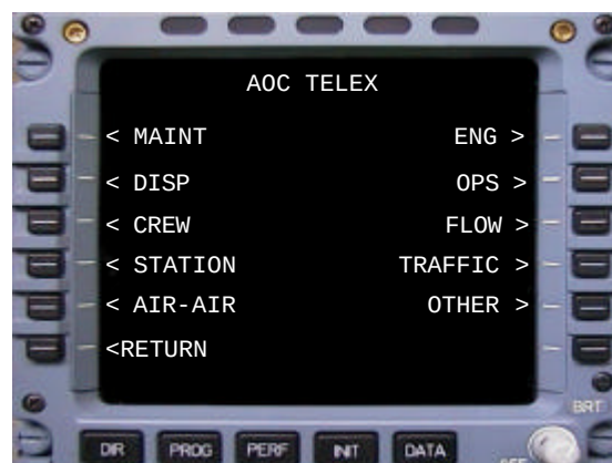
Figure 4.2: Example of AOC Telex MCDU page
