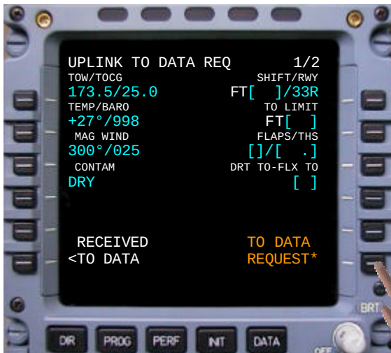
Figure 4.6 Example FMS ACARS TODC request screen
