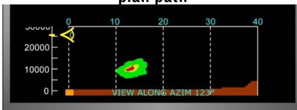
Figure 7-41: VD image on manual selected azimuth
