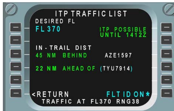
Figure 3-24: ITP possible with detected non-ADS-B aircraft
