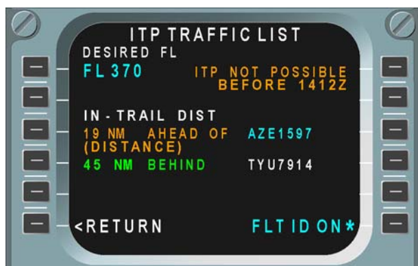
Figure 3-25: ITP not possible due to the distance with one aircraft
