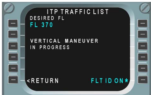
Figure 3-28: ITP in progress
