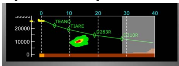
Figure 7-40: VD image on FMS flight plan path
