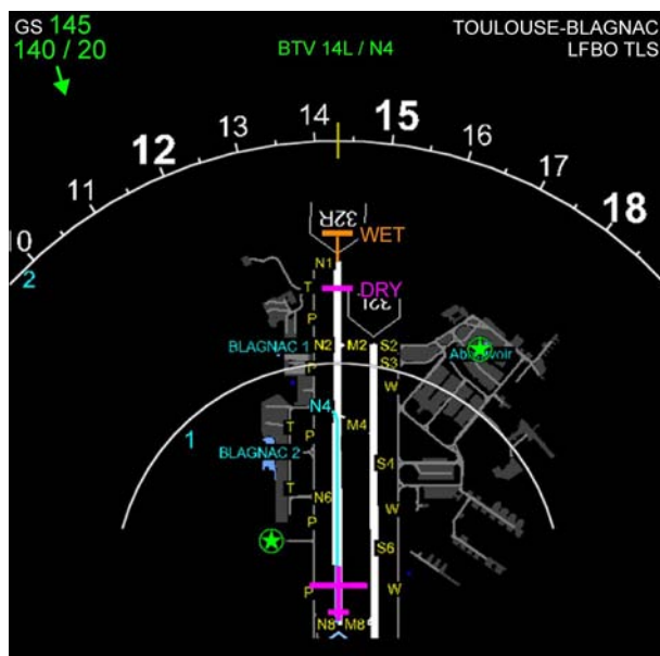
Figure 5-24: ND – ROW engaged with BTV selected (wet conditions)
