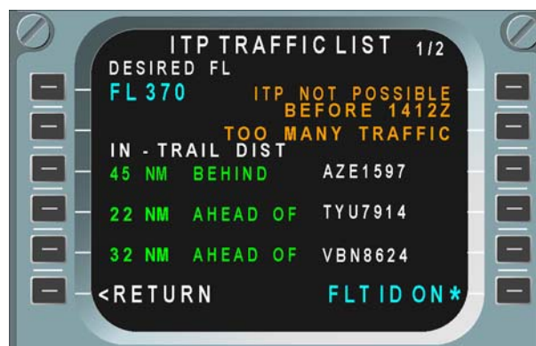
Figure 3-26: ITP not possible due to the number of aircraft
