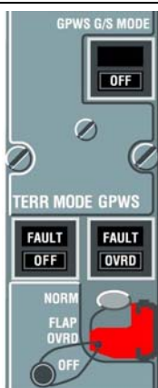
Figure 4-21: Control panel on Captain side
