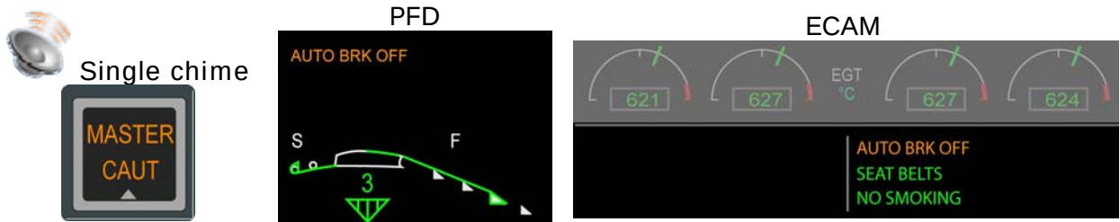
Figure 5-32: Indications for inadvertent or automatic auto brake disconnection
