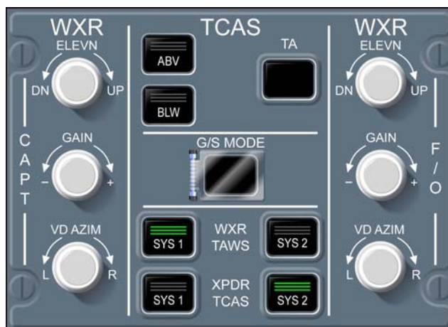
Figure 7-46: AESS Control Panel
