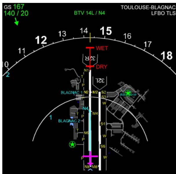
Figure 5-26: ND – ROW engaged with BTV selected (dry conditions)
