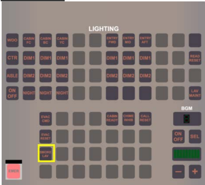
Figure 4-9 Lavatory Smoke Indications
