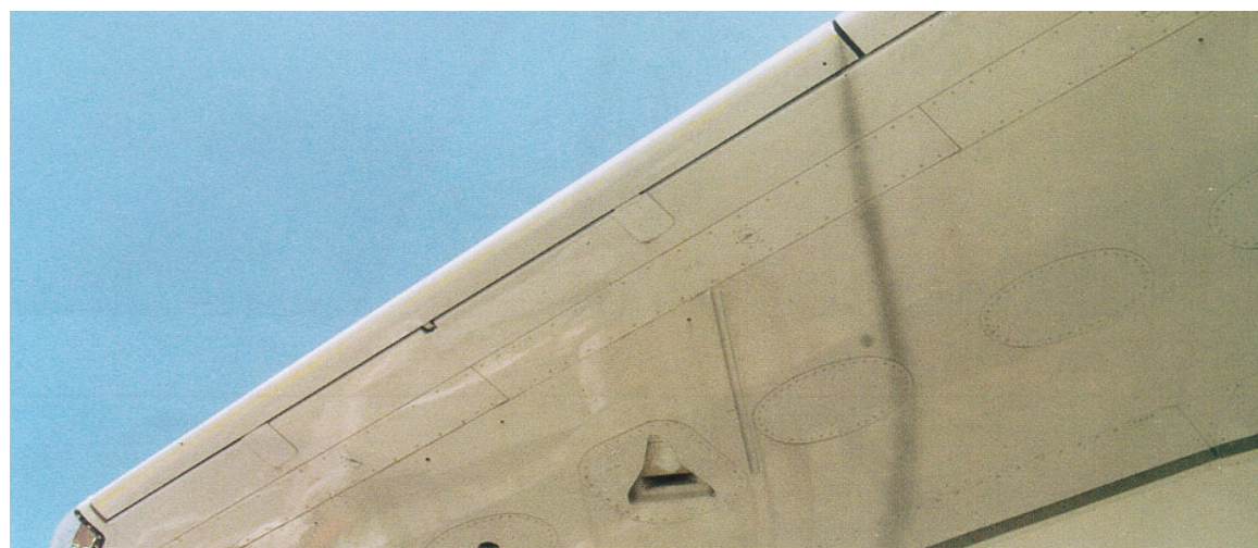
Missing chordwise seal
