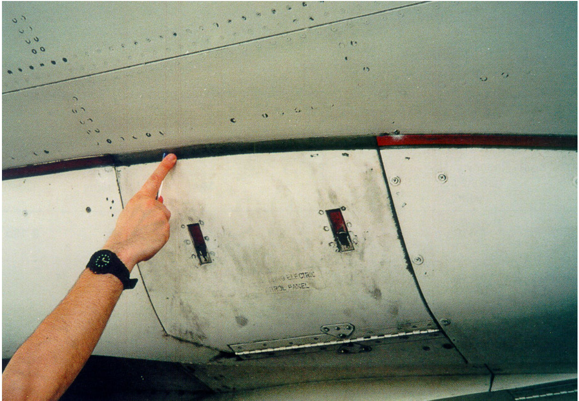
Missing service door seal
