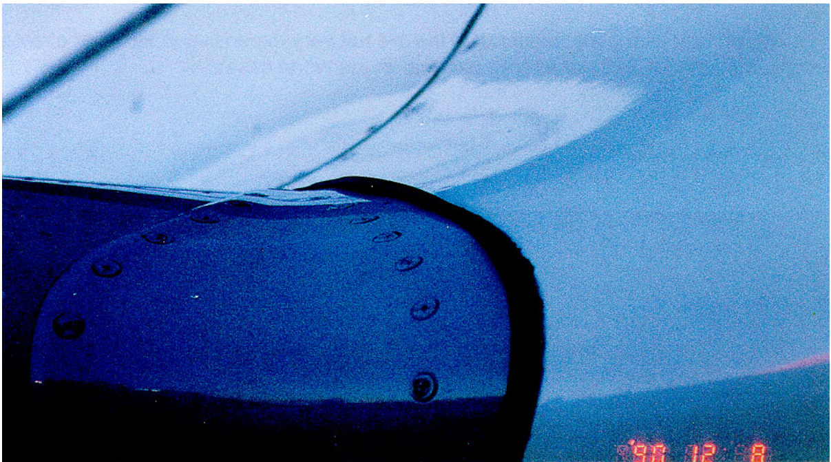
Overfilled seal on the wing / belly fairing junction
