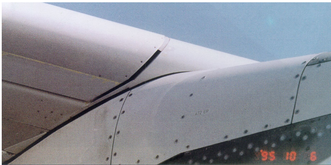
Missing chordwise seal
