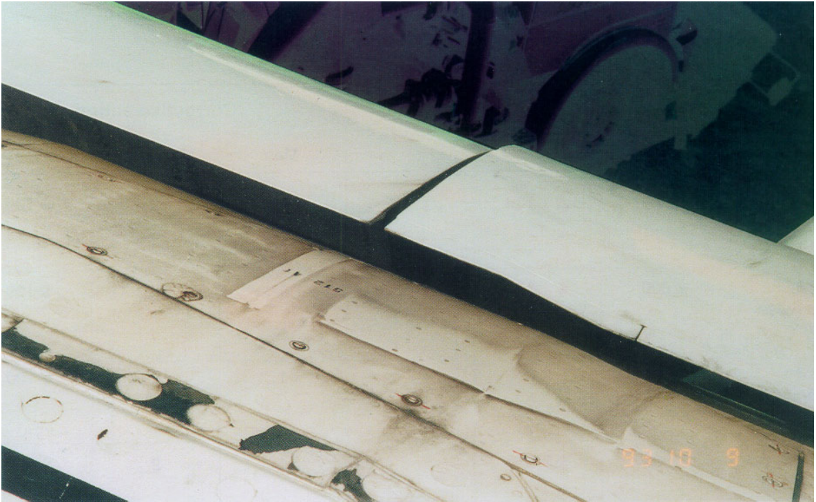
Absence of spanwise slat seal
