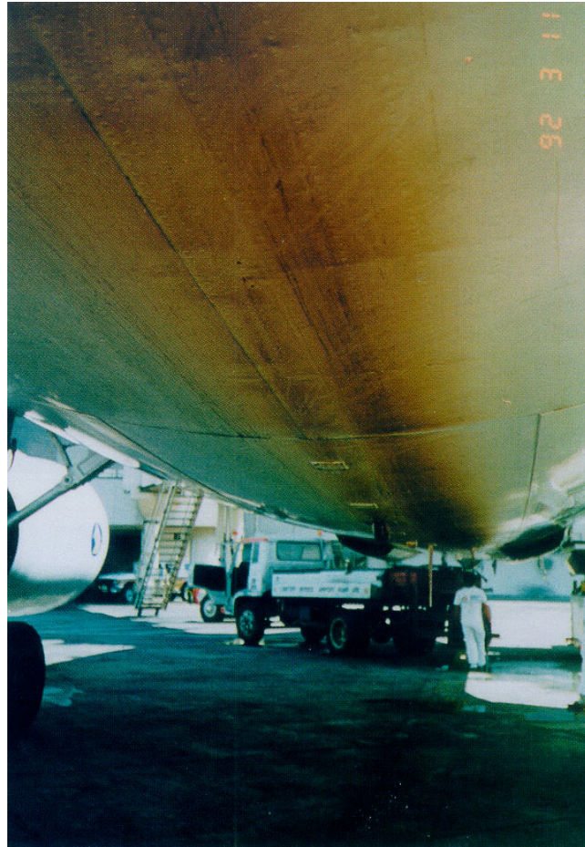
Roughness surface due to skydrol leakage on the belly fairing
