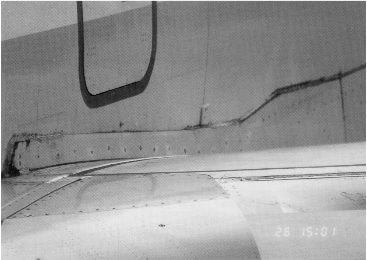
Overfilled belly fairing butt joint gaps
